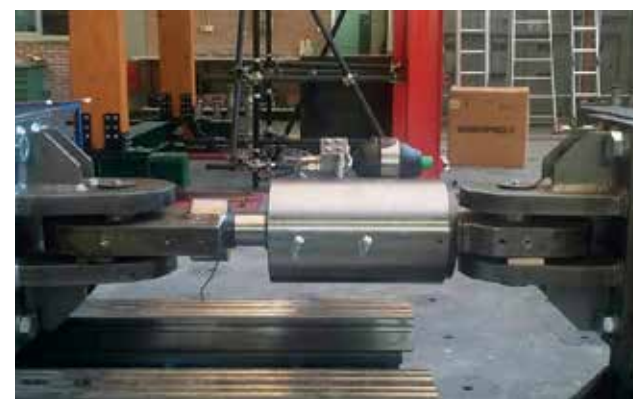
Type Test on TFVD device
